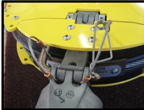
Properly Closed Gate Figure 10
