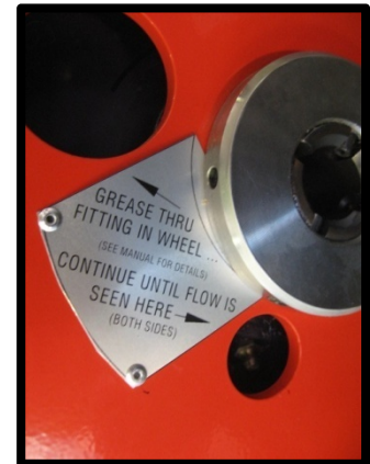
Greasing Holes Figure 12
