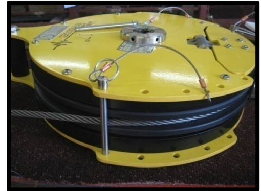
Properly Closed Gate Figure 11
