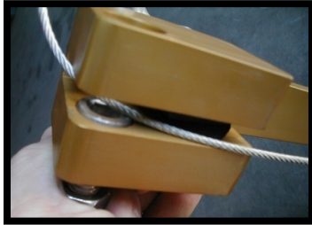
Loading the Slickline, Figure 19
