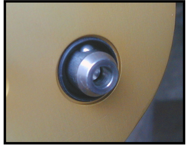
Secured Ball-lock Figure 16
