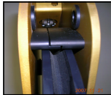
Cable shrouds reduce "line jump"
